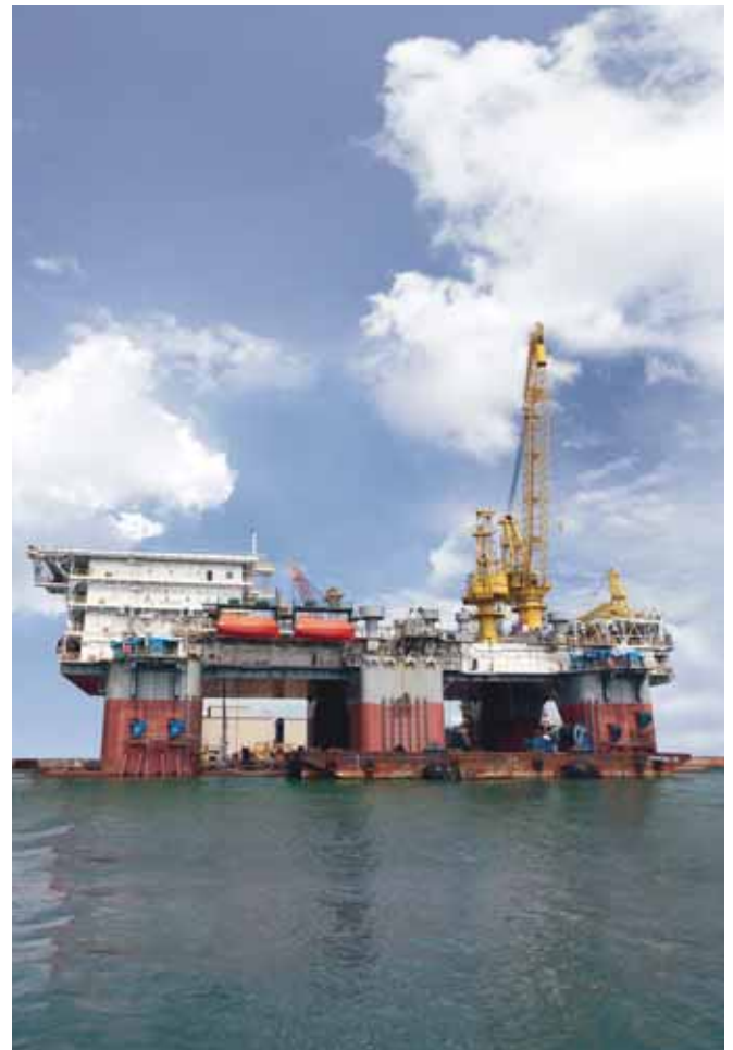
Developed by Keppel's Deepwater Technology Group, the KFELS SSDT™ has revolutionised the way in which drilling tenders operate, allowing them to be deployed next to deepwater floating platforms for the first time.
