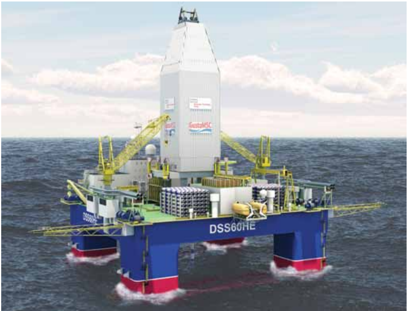
Developed for operating in harsh environments such as the North Sea, the DSS TM 51HE and DSS TM 60HE (in image) designs include winterised features such as derrick cladding and machinery space heating.
