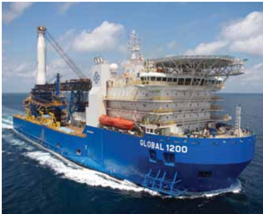
Product of a winning partnership and excellent project management, GLOBAL 1200 is a new generation derrick pipelay vessel built by Keppel Singmarine for Global Industries.
