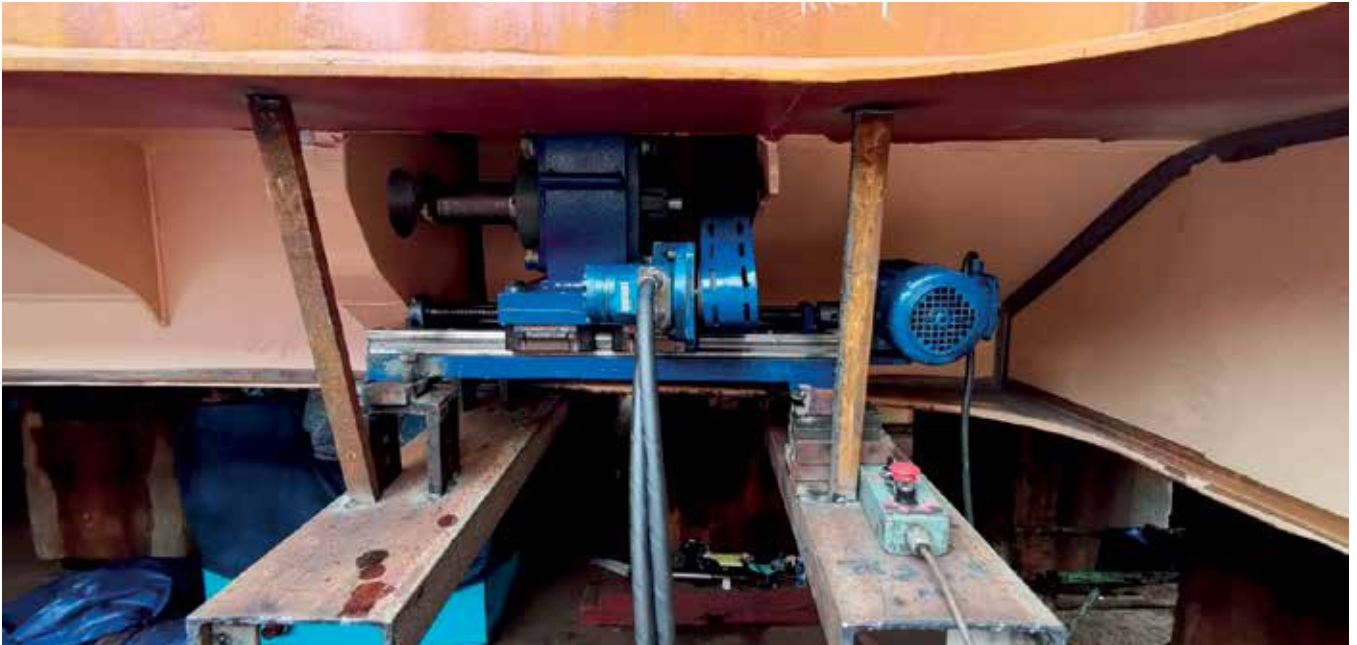
Compared to previous machines, PRISM weighs 90% lighter at 200 kilogrammes, and is 70% smaller at 1.2 metres long, making it more portable and easier to be deployed
