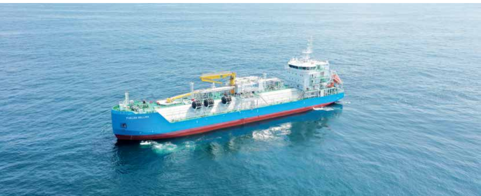
Designed and built by Keppel O&M, the FueLNG Bellina is Singapore's first LBV as well as the world's first bunkering vessel with smart notation
