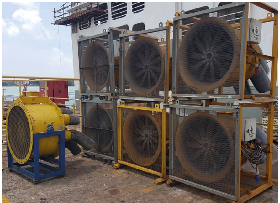
Keppel Shipyard modified the design of ventilation blowers and saved some 14,400kWh of energy per year.
