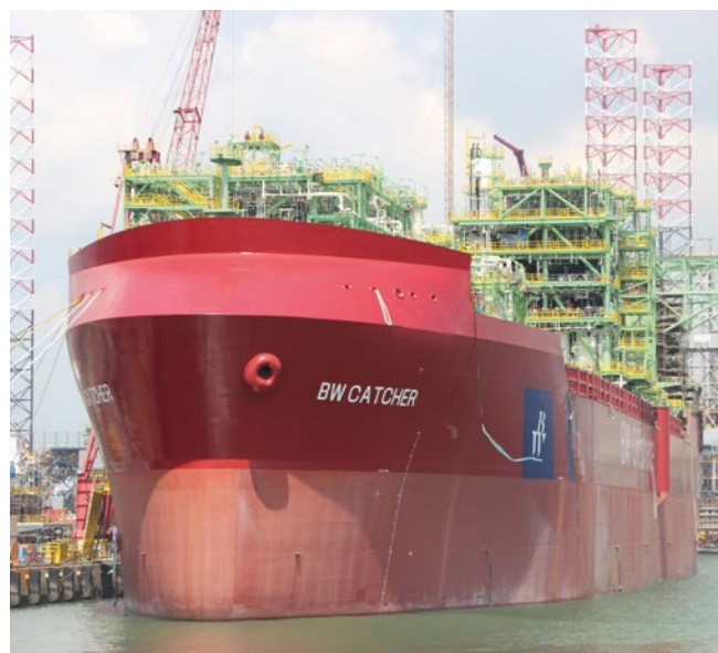
Keppel O&M secured four FPSO projects in 2016, including the topsides installation and integration on the BW Catcher.
