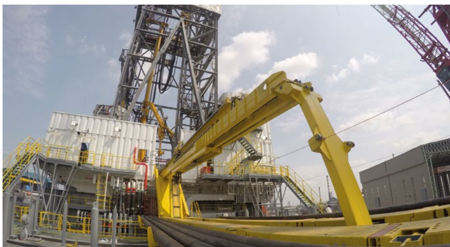
The hydraulic catwalk (pictured) installed on a KFELS B Class jackup rig offers best-in-class cycle times for moving drill pipes and tubulars from the pipe storage area up to the drill floor.
