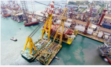
Four floating cranes support the lifting capabilities of the yards in Singapore:
