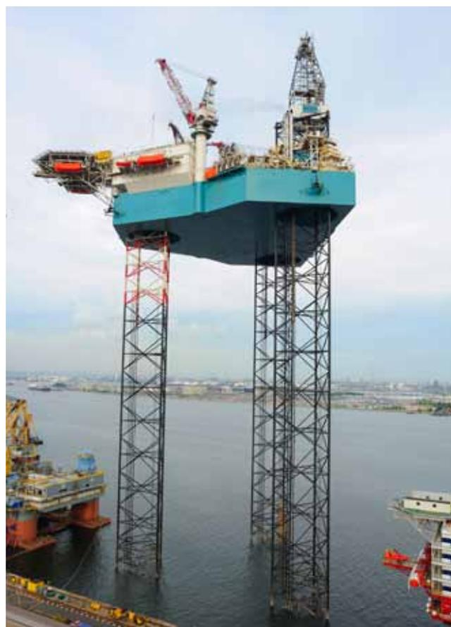
Keppel has delivered to Rowan companies three KFELS N Class jackups. The design is in full compliance with requirements for rigs operating in the Norwegian sector of the North Sea
