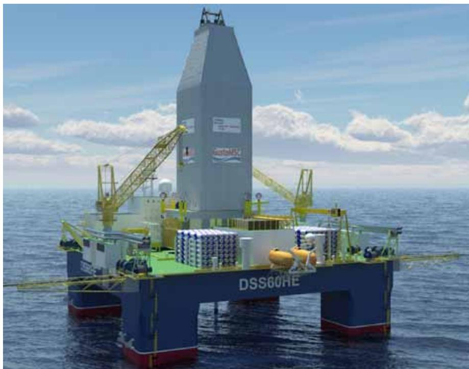
Equipped with winterised features such as derrick cladding and machinery space heating, DSS™51HE and DSS™60HE (pictured) semis are capable of year-round operations
