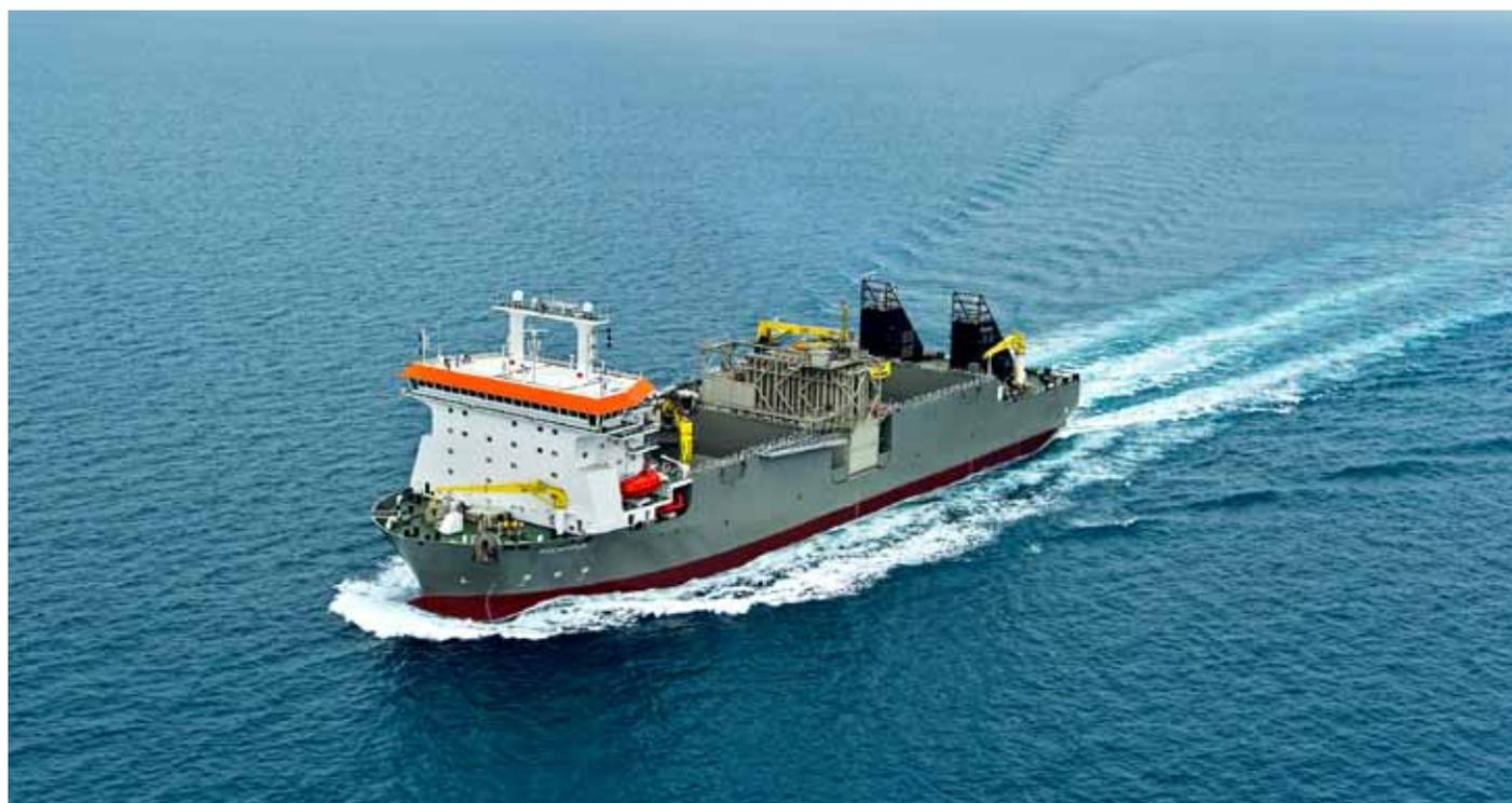
Rockpiper is a rock dumping fall pipe vessel built by Keppel Singmarine for the Dutch company Boskalis
